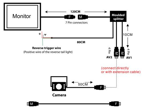
Video Extension cable (used between camera and AV2)  $\frac{7M}{10M}$  optional
